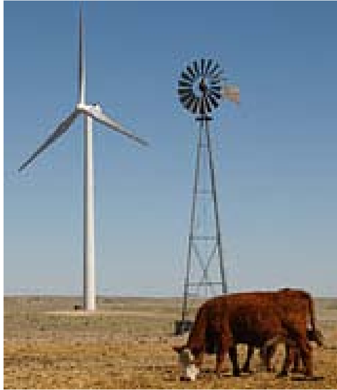
Fig. 1: Aerodynamic and impulse or drag horizontal axis wind turbines.
