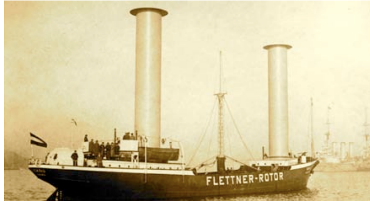
Fig. 35: Magnus Flettner rotor equipped ship first named Buckau then renamed Baden-Baden. Source: Popular Mechanics.
