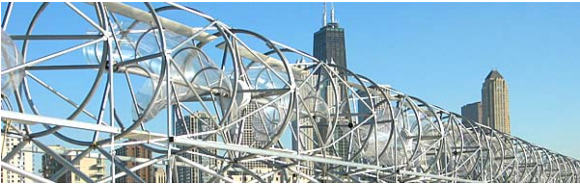
Fig. 61: Horizontal helical turbine.
