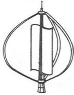
Fig. 8: Combined Darrieus and Savonius vertical axis wind turbine.
