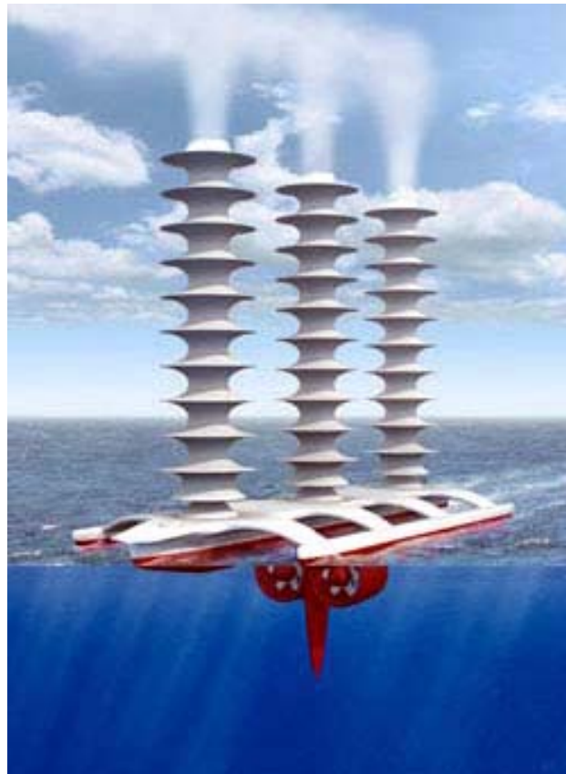
Fig. 41: Conceptual design of cloud seeding autonomous ship with Thom rotors.
